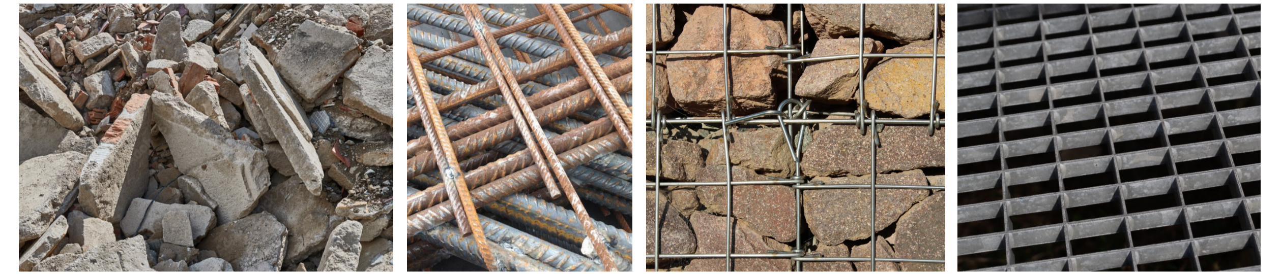
Gabion system that serves as foundations for the pavilion. No anchors on the ground are needed. rubble, steel rods for reinforced concrete, gabion cage...
